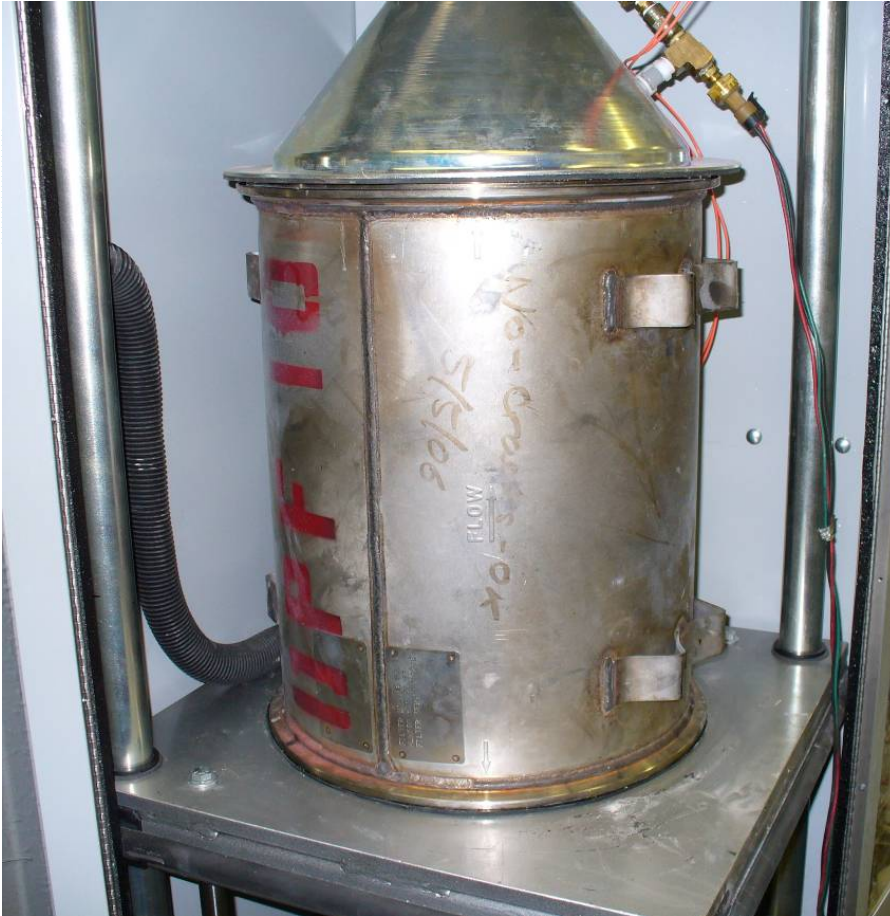
A Detroit Diesel 13" DPF clamped in position for cleaning.
